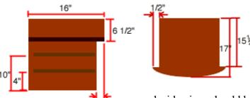
Firstly, the two side pieces should be cut to shape in the following way. The front edge of
